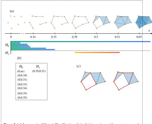
Figure 1 (a) An example of Vietoris-Rips filtration of simplicial complexes with parameter  $\varepsilon$ , and the corresponding barcode for 0- and 1-dimensional persistent homology. (b) The persistent pairs of the above filtration. (c) Two equivalent representatives of the (only) generator of  $PH_1$ .
