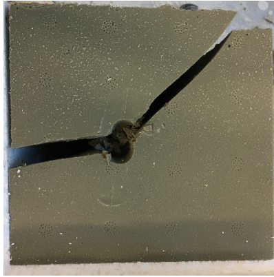
Figure 55 - Cubic sample (150*150*150 mm) of two-component grout, demoulded, tested with the penetrometer. Test failed.
