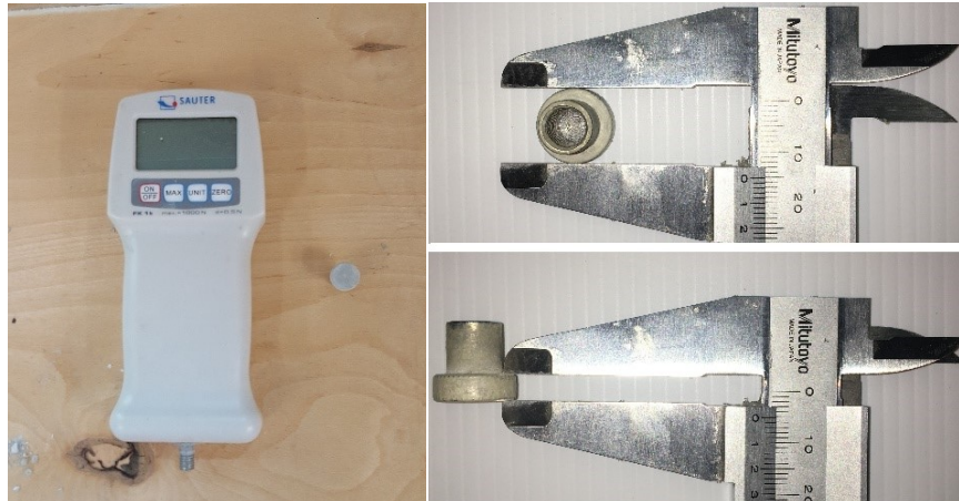
Figure 50 - SAUTER GmbH Ziegelei 1 D-72336 Balingen digital model dynamometer (left) and bit details (right).
