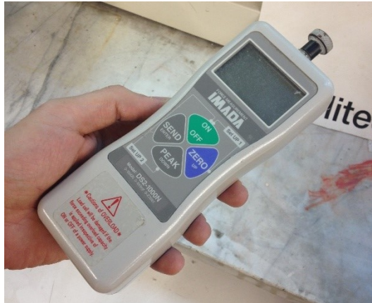
Figure 49 - IMADA DS2-1000N used for the penetrometer assessment.
