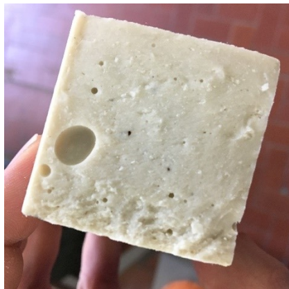
Figure 41 - Example of a big air bubble trapped inside the medium, close to the casting surface. Sample discarded.
