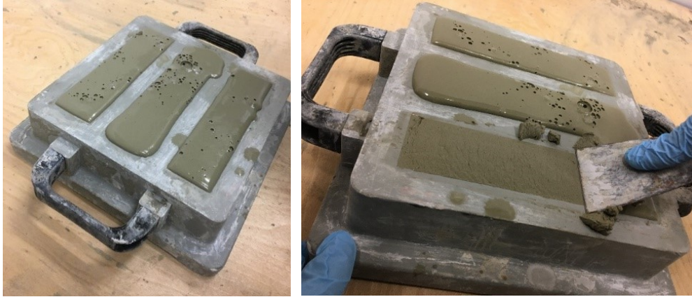
Figure 42 - Samples cast calculating a bigger total volume of components. Bubbles are clearly visible on the cast surface (left). Samples trimming performed with a spatula (right) allows the removal of the potential weak points due to the presence of bubbles.
