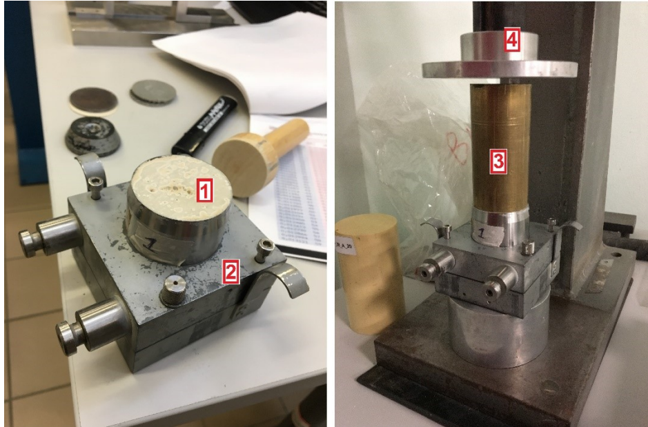
Figure 60 – Sample of two-component grout in the mould (left) and transferring phase of the sample from the mould into the shear box (right).
