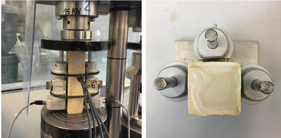
Figure 77 - Extensometers applied on a two-component grout sample before testing.
