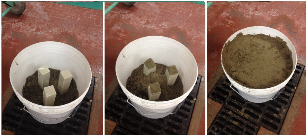
Figure 94 - Samples cured in sand. Photos of the burial phase.
