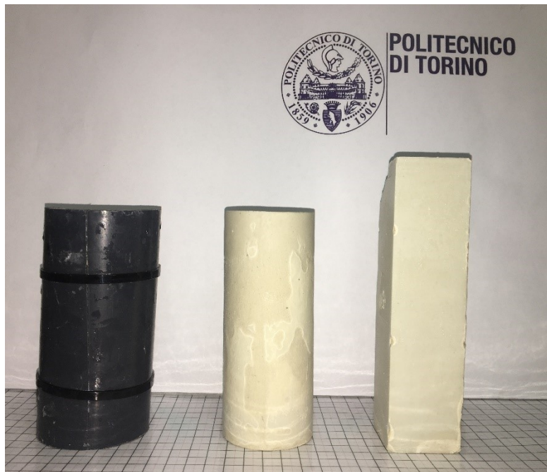
Figure 85 - From left to right: the cylindrical mould used, cylindrical and prismatic two-component grout samples. The background unit scale is 1 cm.
