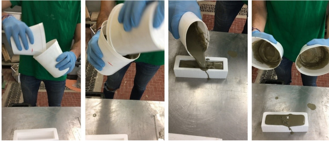
Figure 40 - From left to right: component A poured into the component B tank, the mixed grout poured again into the previous tank and eventually the sample casting. In the last photo the residual material on the inner tank surfaces can be observed.
