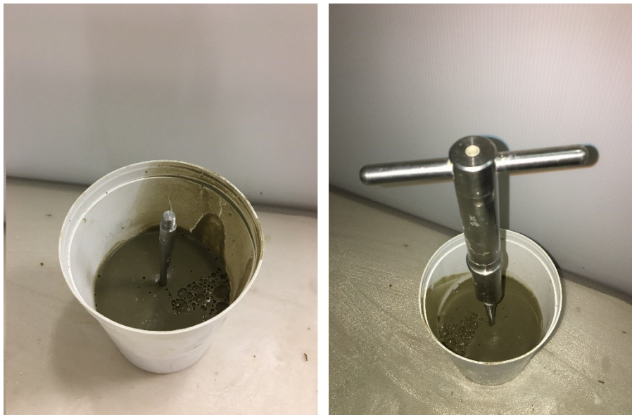
Figure 74 - The vane pre-installed in the grout (left) and the assembled vane test device just before testing (right).
