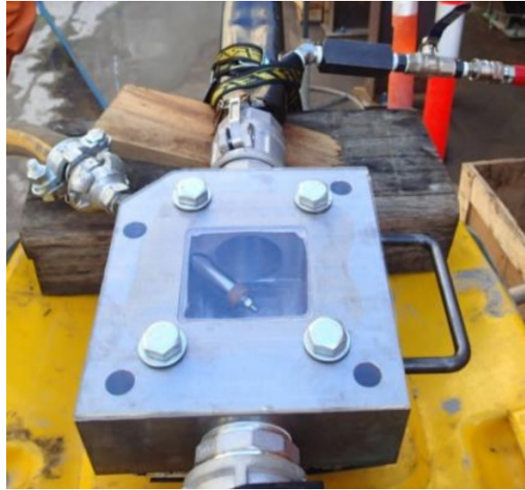
Figure 25 - Trial grout mix box. On the top the component mixer is depicted (Ivantchev & Dal Rio, 2015).
