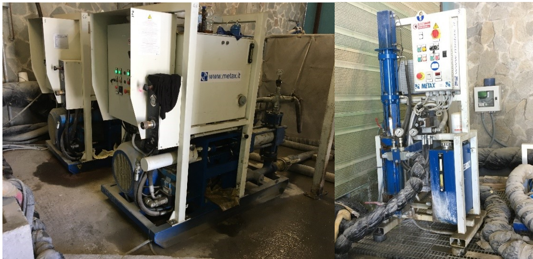
Figure 18 - Double piston pump for the component A transportation (left). Single piston pump for the component B transportation (right).
