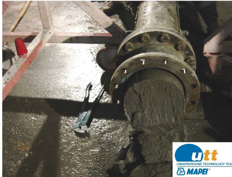
Figure 23 - Component A tube choking. The photo is property of the UTT Mapei. (Richard Schulkins master lecture, 2020).
