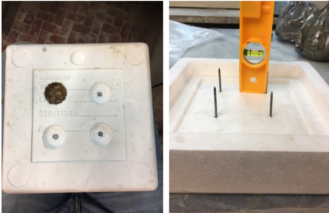
Figure 111 - Polystyrene support used for the samples production.
