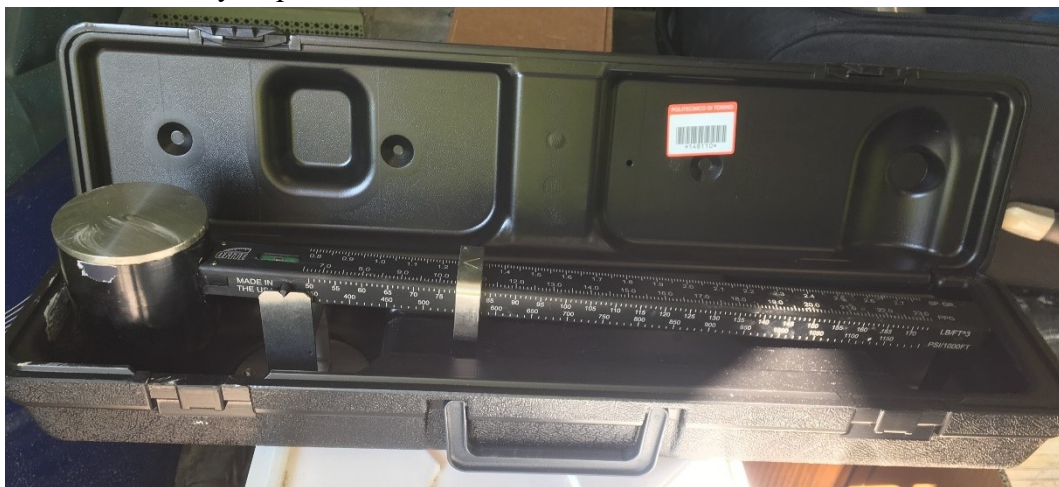
Figure 36 - Mud balance used.
