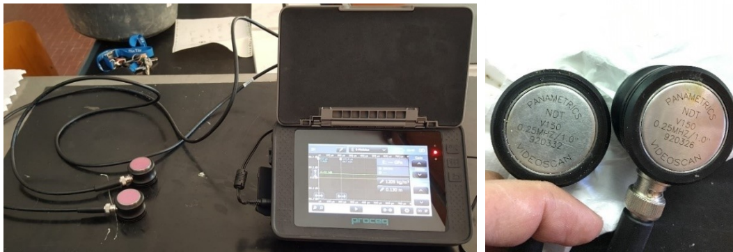
Figure 83 - Picture of Pundit® PL-200 (left) and the transducers used with a natural frequency of 250 kHz (right);
