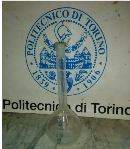
Figure 37 - 250 mL volumetric flask used for the component A unit weight assessment.
