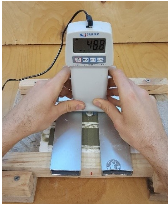
Figure 52 - Penetrometric testing phase. In this specific case, the mould in polystyrene is locked by the wood block device. The mould displacements are constrained. The steel guide leads the bit penetration to the wanted length.
