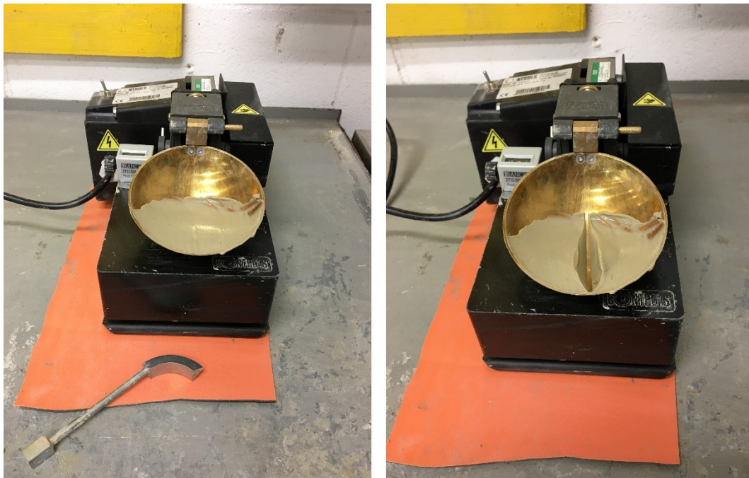
Figure 122 - Casagrande apparatus with the cup filled with a sample of bentonite 1 and grooving tool (left). Casagrande apparatus with the groove in the centre, just before starting the test (right).
