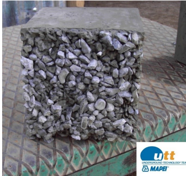
Figure 10 - Sample of pea gravel after a cement mortar secondary injection. The photo is property of UTT Mapei. (Richard Schulkins master lecture, 2020).
