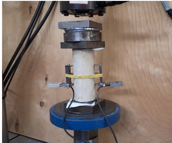
Figure 82 - Cylinder sample and transducers for the elastic modulus assessment. System discarded because of adhesion problems.
