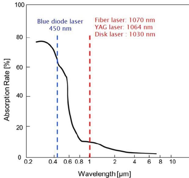
Figure 1. Absorption rate in copper for different wavelengths.
