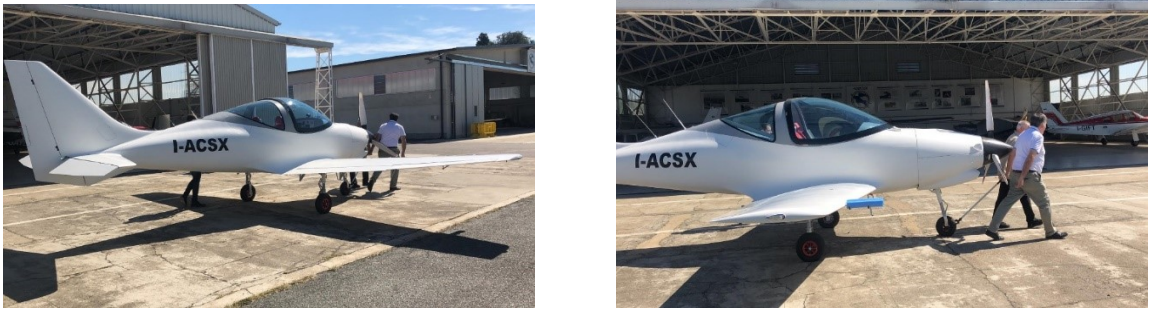
Figure 30: OMA acquisition during taxing vibration test.
