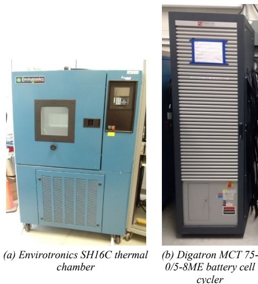
Fig. 7. Battery test equipment for ageing test
