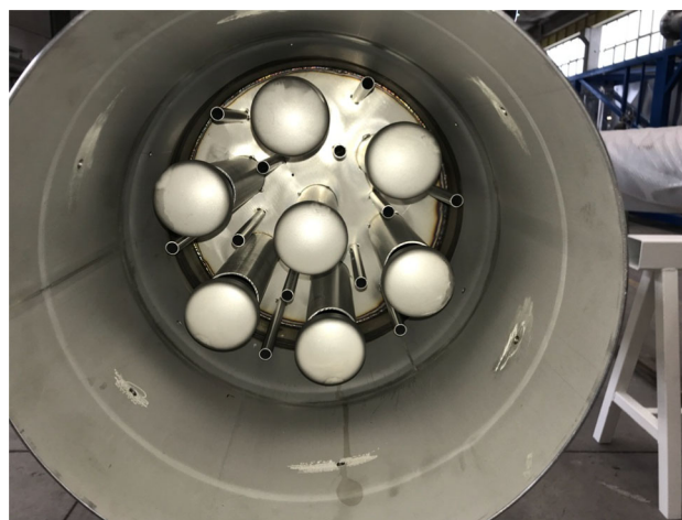
Fig. 7 A view from above of a liquid distributor. The small pipes without a top cap are perforated on the side, allowing the liquid to flow down to the column section below. The wider pipes with the top cap are the chimneys allowing the vapor to rise from the column section below
