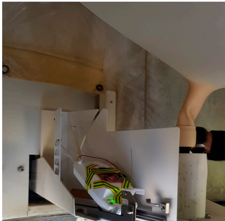
Figure 5. System setup 2 used to determine the transmission ranges reached by the radioprobe system in an open-area environment. Tiny radioprobe attached to the reference atmospheric sounding system.
