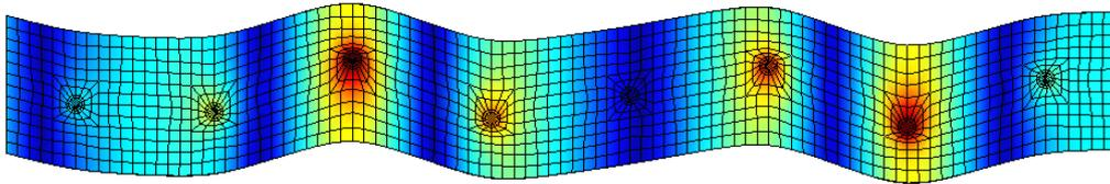
(c) Shear wave - 792 Hz
