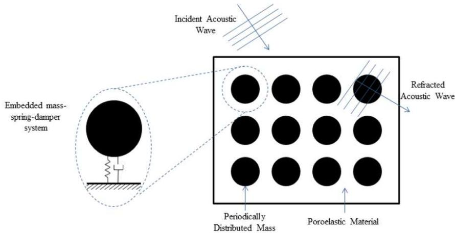
Figure 1: Heterogeneous metamaterial panel with cylindrical through-the-thickness inclusions.
