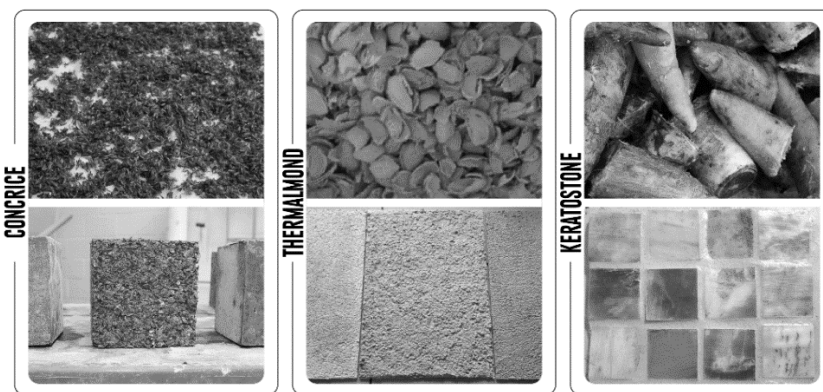
Figure 1.1 Specimens manufactured from agricultural by products and waste. From left to right: Concrice; Thermalmond; Keratostone.
