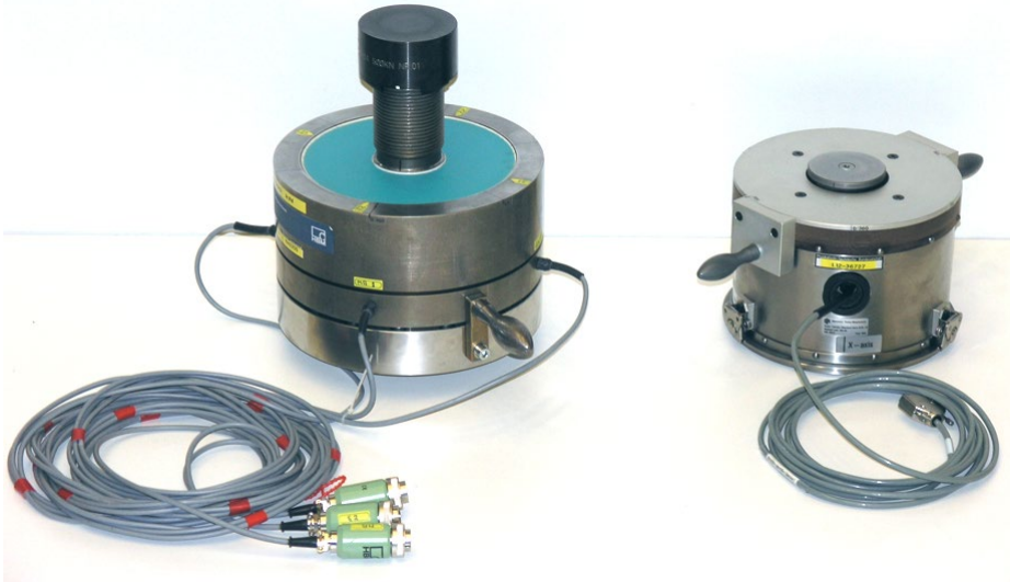
Figure 3: Photograph of the two 500 kN force transducers
