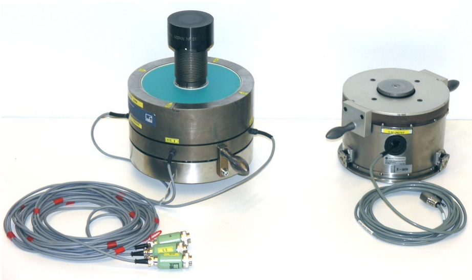
Figure 3: Photograph of the two 500 kN force transducers
