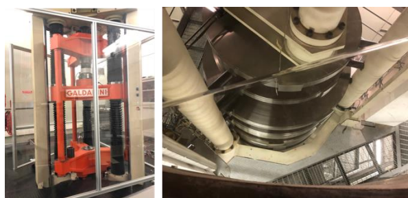
Figure 1: The 1 MN deadweight force standard machine
