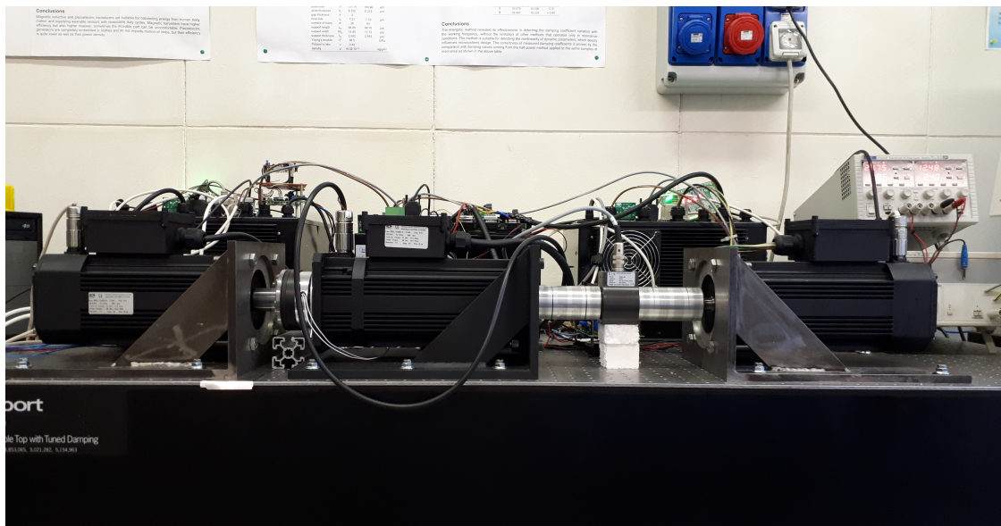
Figure 7. (a) Hardware in the Loop bench layout, (b) test bench.
