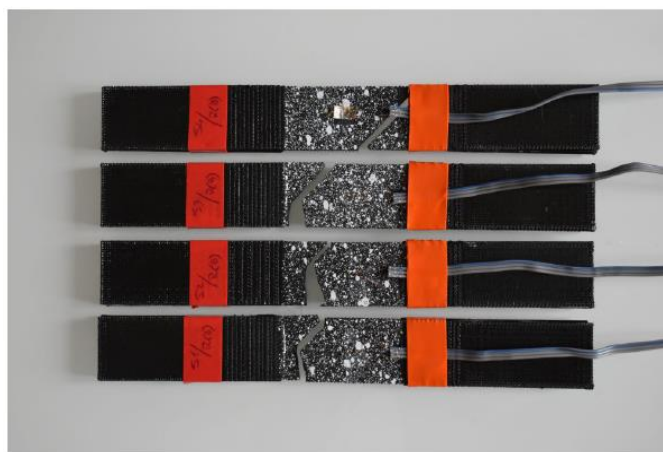
Fig. 7: Run(B) specimens after the tensile test ended
