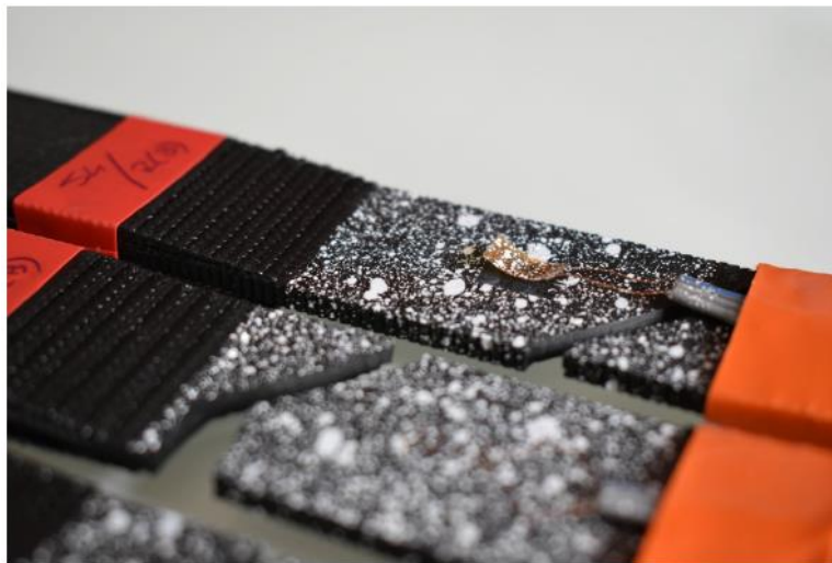
Fig. 14: Run(B) I4 specimen: the strain gauge detached from the specimen during the tensile test
