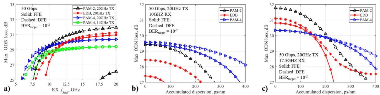
**Fig. 3** a) 50 Gbps simulated maximum ODN loss as a function of the RX  $f_{3dB}$ , considering an optical TX with  $f_{3dB} = 14$  or 20 GHz ( $L=20$ km). b) and c) Maximum ODN loss versus accumulated dispersion for a 20GHz TX in combination with a 10GHz RX or a 17.5GHz RX, respectively.
