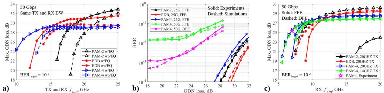
**Fig. 2** a) Maximum ODN loss as a function of the TX and RX -3dB BW for different formats, comparing non-equalized and FFE-equalized cases, in optical BtB. b) Comparison of experimental and simulation BER versus ODN loss results for different modulation formats and bit rates [5] ( $L=20$ km). c) 50 Gbps simulated maximum ODN loss as a function of the RX  $f_{3dB}$ , considering optical TX with  $f_{3dB} = 14$  or 20 GHz ( $L=20$ km)
