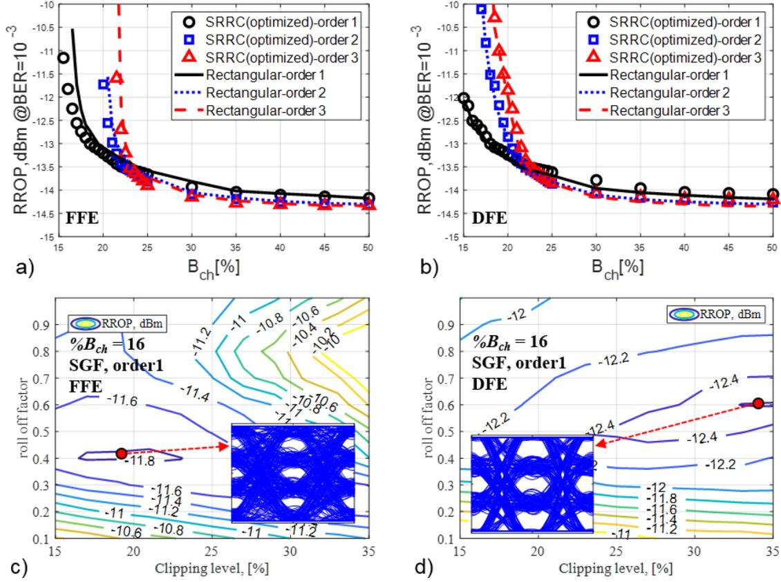
Figure 2. Required ROP as a function of normalized TX and RX BW (%B<sub>ch</sub>) for different TX scenarios using a) FFE, b) DFE. RROP contour plots as a function of SRRC roll-off factor and clipping level (using SGFs n=1), for a %B<sub>ch</sub>=16%, using c) FFE, d) DFE. Inset: Normalized x<sub>DAC</sub>(t) eye-diagrams for optimum point of operation.
