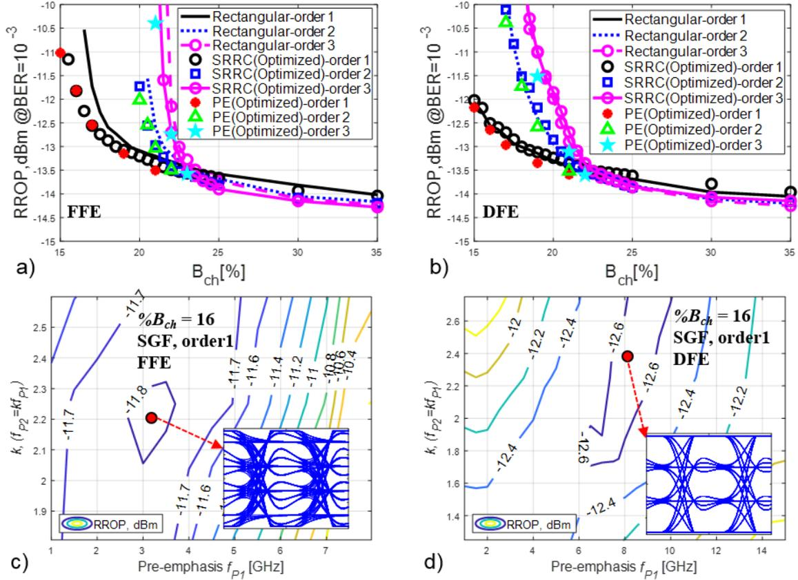
Figure 3. Required ROP as a function of normalized TX and RX BW ( $\%B_{ch}$ ) for different TX scenarios using a) FFE, b) DFE. Pre-emphasis case RROP contour plots as a function of the filter parameters  $f_{p1}$  and  $f_{p2}$ , for a  $\%B_{ch}=16\%$  and optimized clipping level  $CL = 25\%$  (using SGFs of order 1 for TX and RX O/E), using c) FFE, d) DFE. Inset: Normalized  $x_{DAC}(t)$  eye-diagrams for optimum point of operation. PE: Pre-Emphasis.
