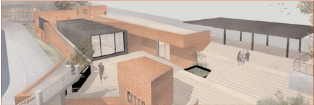
Figure 6 Solution for the urban connection. Redefinition of the public space and arrangement of vertical connections; view on the new sports building ( elaboration by the authors )
