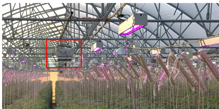
Figure 5. Sensors installed inside the greenhouse with the electrical cabinet containing the data monitoring unit hung to the greenhouse cover.
