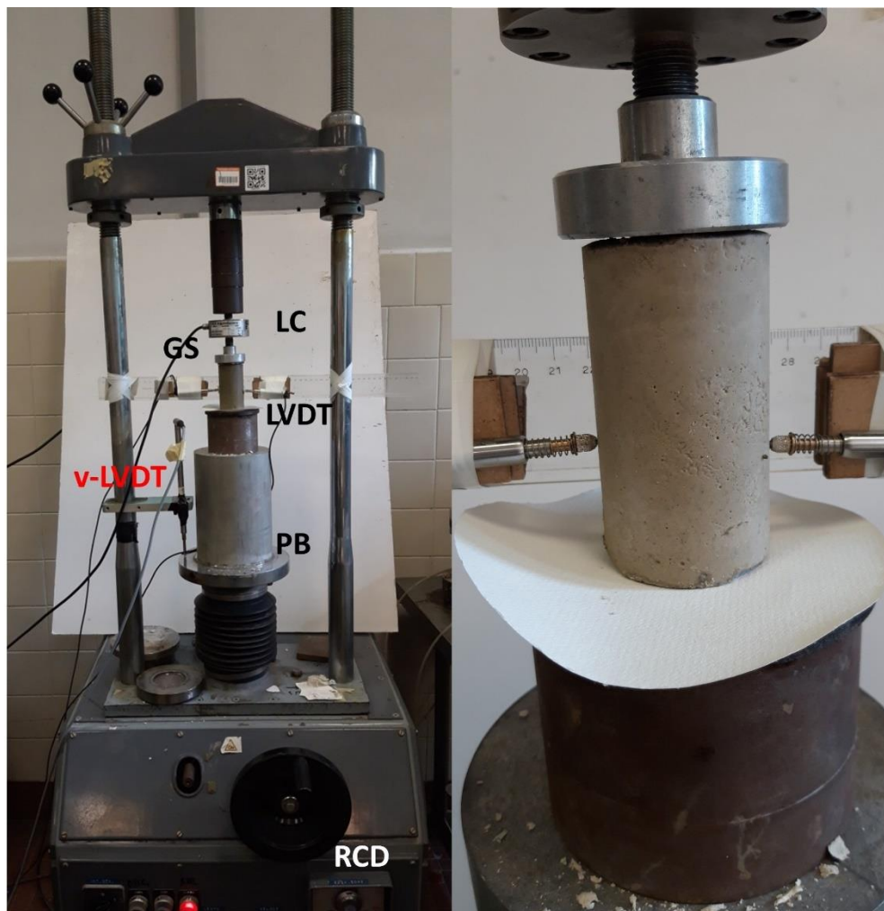
236 Fig. 2 Testing equipment for compression (left) and enlargement of the UCS sample 237 (right). LC: load cell; GS: grout sample; LVDT: radial coupled LVDT transducers; 238 vLVDT: vertical LVDT transducer; PB: base of press plate; RCD: device for advance 239 rate control.
