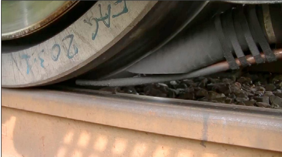
Fig. 3. System used to spread the soap on the rail during the experimental tests.
