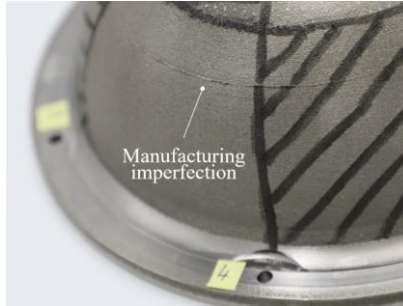
Fig. 11 Manufacturing imperfection. A system of reference was marked on the shells, to help in locating the failures.
