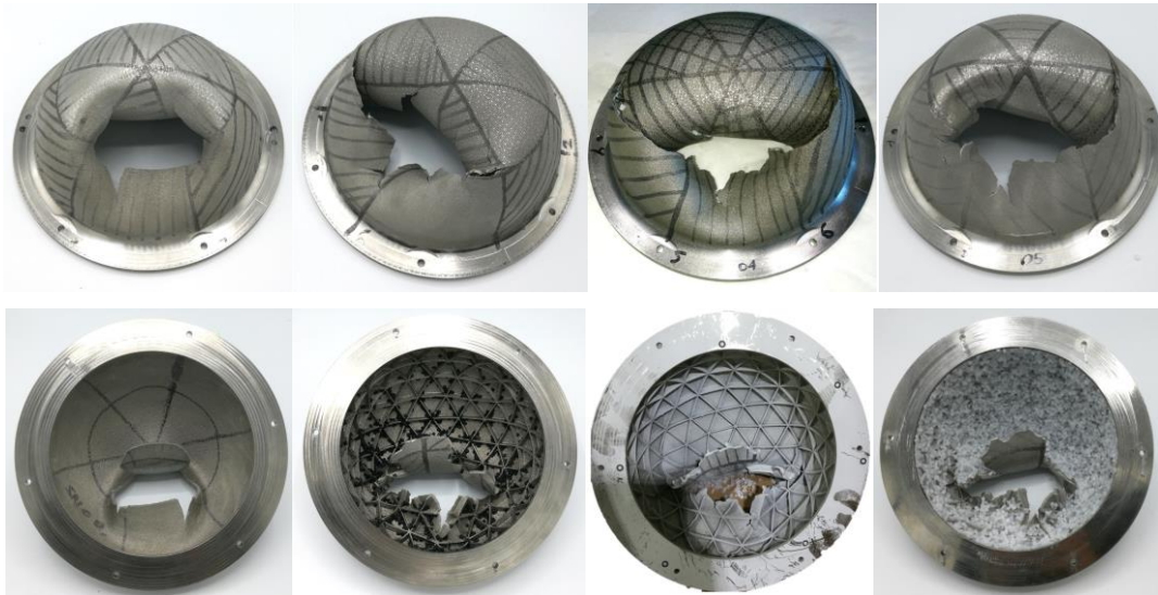
Fig. 13 Tested components: plain-SN00 (first column), isoSN01 (second column), iso-SN04 (third column), iso-SN05 (fourth column).
