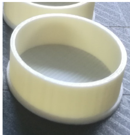
Fig. 1. Mould for suction controlled oedometer test [8].
