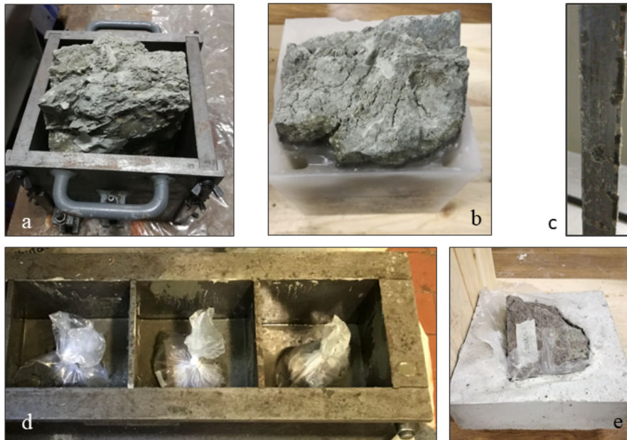
Figure 5.12: a) An irregular melange specimen in the formwork before the paraffin injection; b) the specimen in the paraffin; c) the melted diamond blade after the first cut; d) irregular melange specimens in the formwork before the mortar injection; e) a melange specimen in the mortar.
