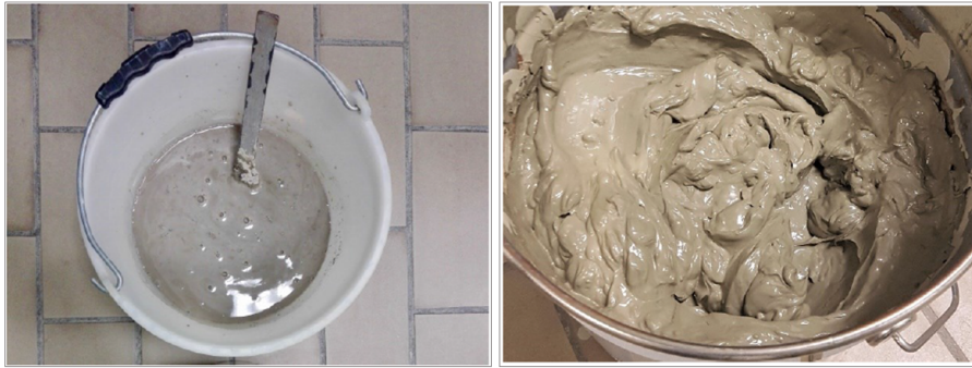
Figure 7.2: Sieved soil mixture inside the plastic container.
