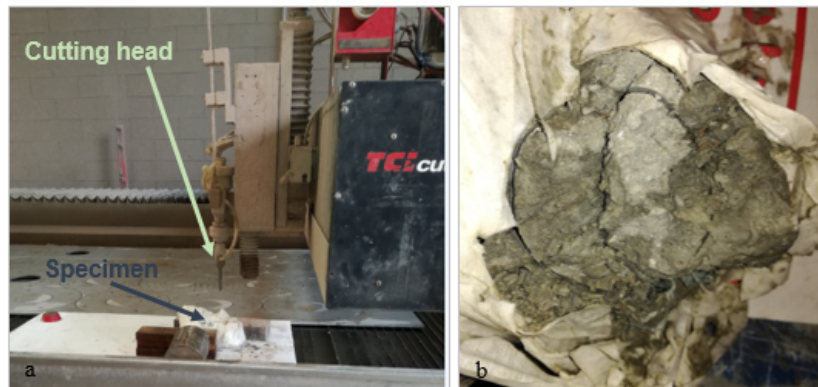
Figure 5.8: a) Waterjet cutting machine and irregular melange lump with side dimensions of about 23x18x13 cm; b) the melange after the cut (OMT S.r.l., Leinì, Torino).
