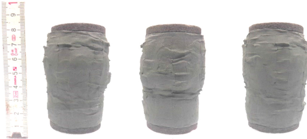
Figure 7.15: Failure modes of the heterogeneous specimen with 50% VBP.
