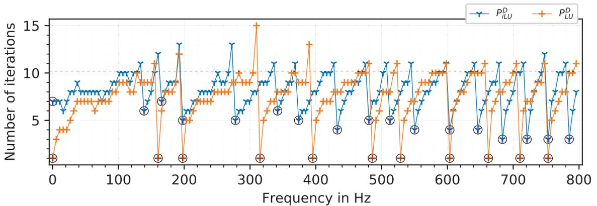
Figure 4: Number of GMRES iterations to convergence when using delayed frequency preconditioners (DFP) algorithm. The delayed preconditioners are incomplete  $\mathbf{P}_{iLU}^D$  and complete  $\mathbf{P}_{LU}^D$ .
