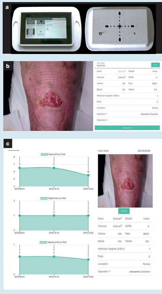
Fig 1. Wound Viewer: on one side the capacitive touch screen is displayed with the user interface, while the other shows the digital camera, the 16 infrared sensor-array and the four white light-emitting diodes (a). An example of the user interface showing the result of an examination (b). An example of the wound statistics page, designed for health professionals to monitor the wound's evolution (c)
