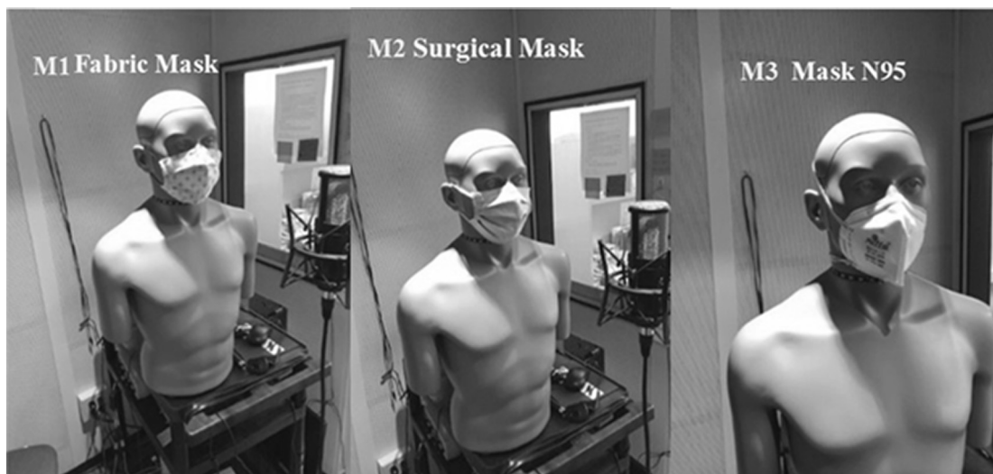
FIG. 1. Head and torso simulator (HATS) wearing the three masks used in the study.
