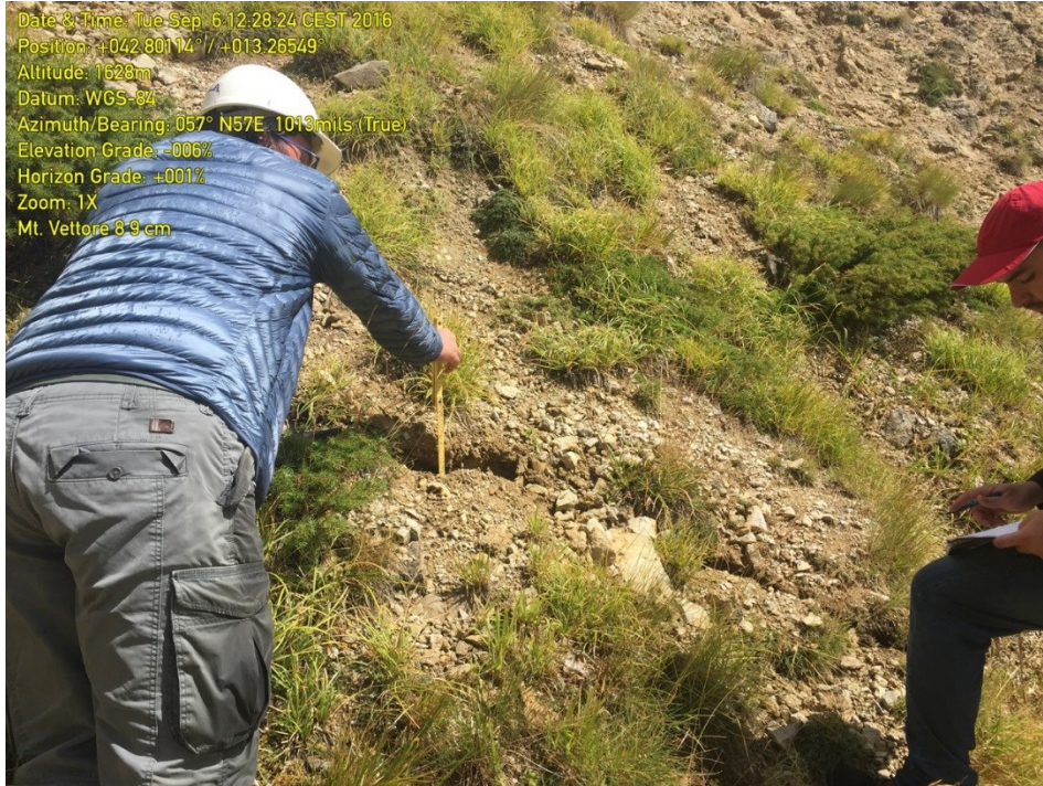
Figure 2.19k. Mt. Vettore fault Site 8 at a WGS84 ellipsoid elevation of 1628 m. The normal fault displacement at this site was 9 cm down toward the west (Latitude and Longitude are annotated on the image).
