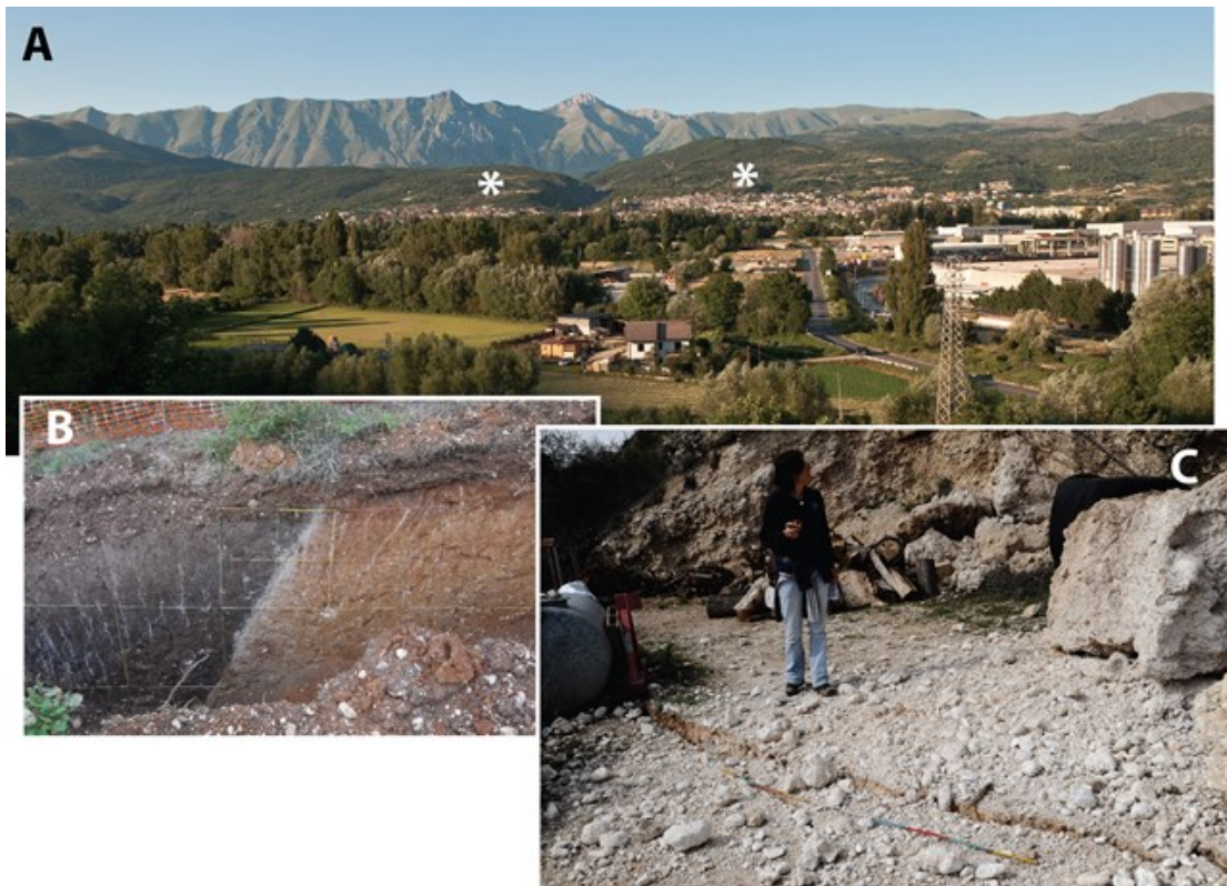
Figure 2.10. a) Panoramic view of the Paganica-Bazzano plain; the white asterisks indicate the gentle slope where the Paganica fault has been detected; b) wall of one the trenches excavated by Moro et al. (2013) across the Paganica fault: the fault places a Pleistocene colluvium (red unit in the footwall) in contact with Upper Pleistocene and Holocene colluvial units in the hanging wall; c) surface faulting observed along the Paganica fault after 6 April 2009 earthquake.
