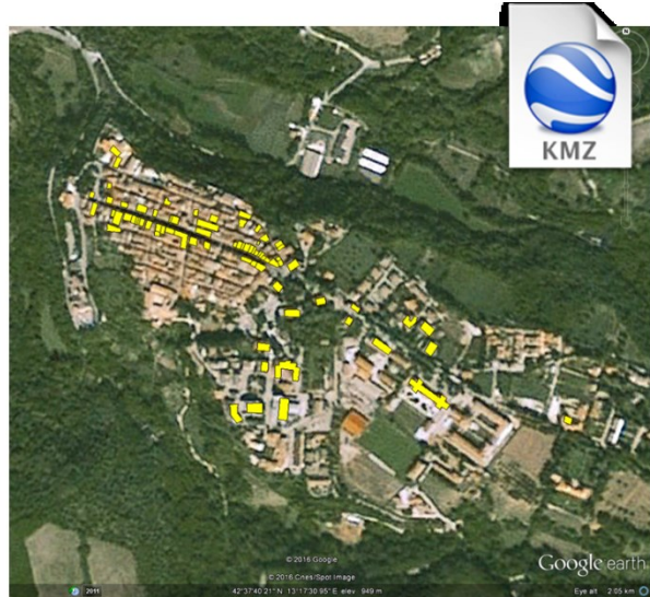
Figure 5.12. Overview of structural damage within the Amatrice Red Zone as seen by aerial image and after visual inspection (note that access to some streets within the Red Zone was not permitted and that additional inspection data are still under post-processing).
