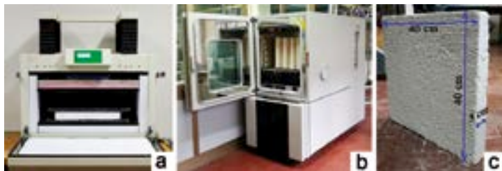
Figure 2 – a) The HFM apparatus for the thermal conductivity and specific heat capacity measurement; b) the climatic chamber adopted for the sample conditioning; c) sample size for the thermal conductivity and specific heat measurement
