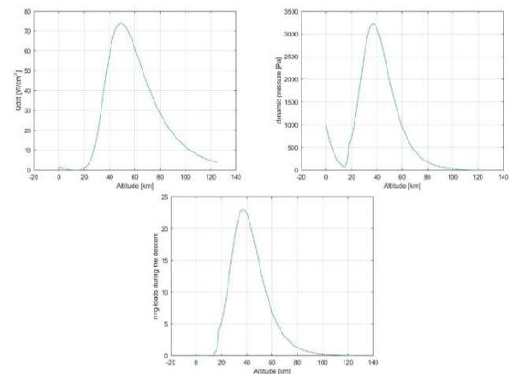
Figure 17: gload, heat flux and dynamic pressure trend
