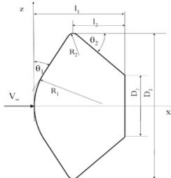
Figure 7: Shape of Beagle-2 heat shield [10]
