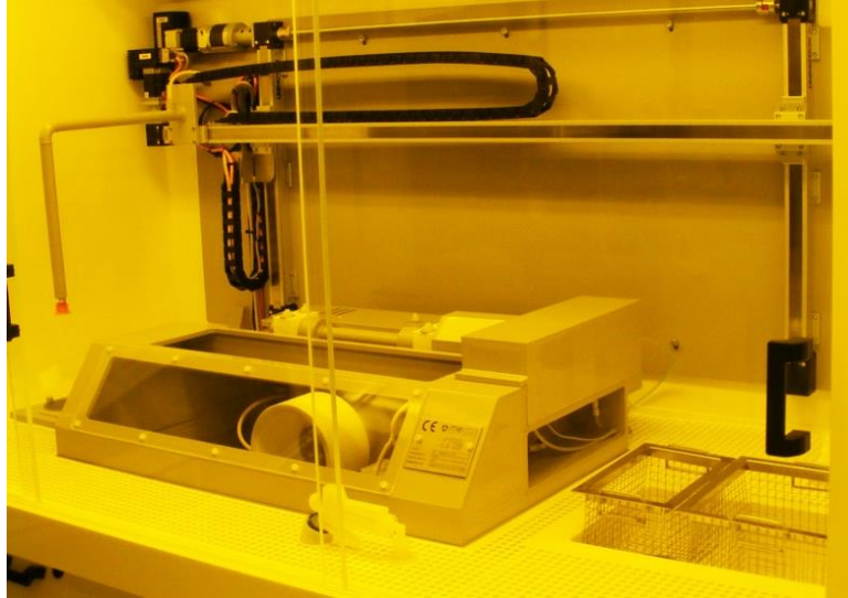
Fig. 3 Automated ELO processing equipment developed at tf2-devices.
