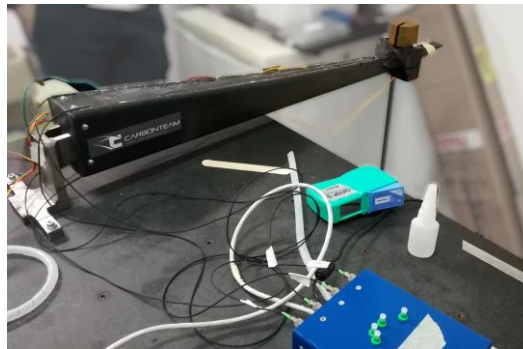
Fig. 4 . Experimental setup for the static load tests on the tail beam
