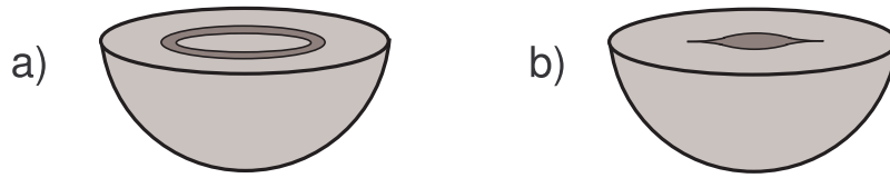
Fig. 1. Basins with circular (a) and straight (b) cracks in ice.
