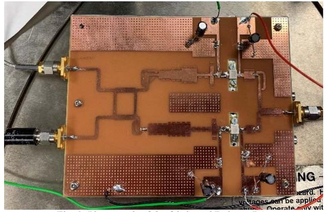
Fig. 2. Photograph of the fabricated Doherty PA
