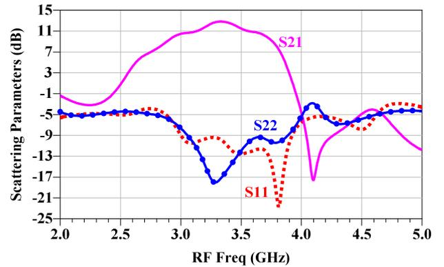
Fig. 3. Simulated S-parameters of the proposed DPA.
