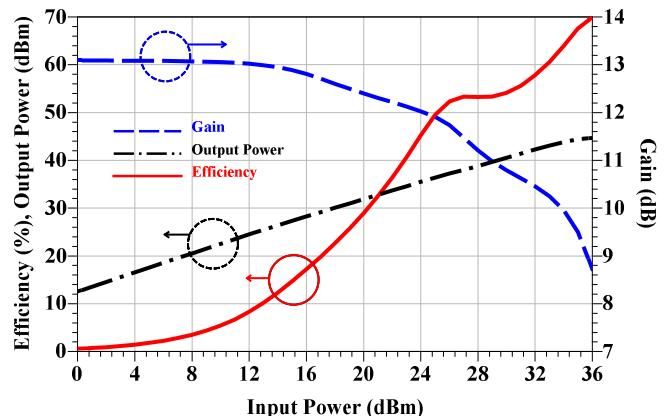
Fig. 4. Simulated DPA performance versus input power at 3.5GHz.
