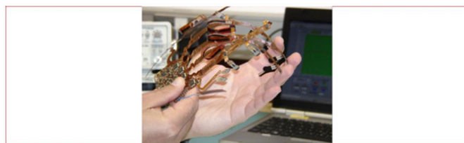
Figure 5 PCB glove under flexion. 14
