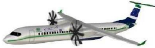
Figure 4: Aircraft with Conventional Configuration (ATR90 and CS-2 Conventional).
