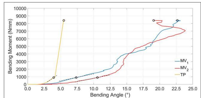
**FIGURE 10 |** Simulation results showing bending moment vs. bending angle. Dashed black lines represent tangent lines used for the  $k_{T900\text{ Nmm}}$  parameter evaluation, while circle markers identify reference points used for  $k_{S900\text{ Nmm}}$  and  $k_{S8400\text{ Nmm}}$  parameters computation (for the sake of clarity secant lines are not reported in figure).
