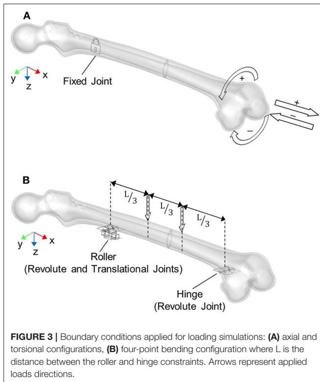
After the nail opening step, three different loads were applied on the bone-fixation device systems:
