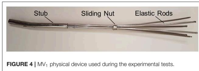
**FIGURE 4** | MV<sub>1</sub> physical device used during the experimental tests.
