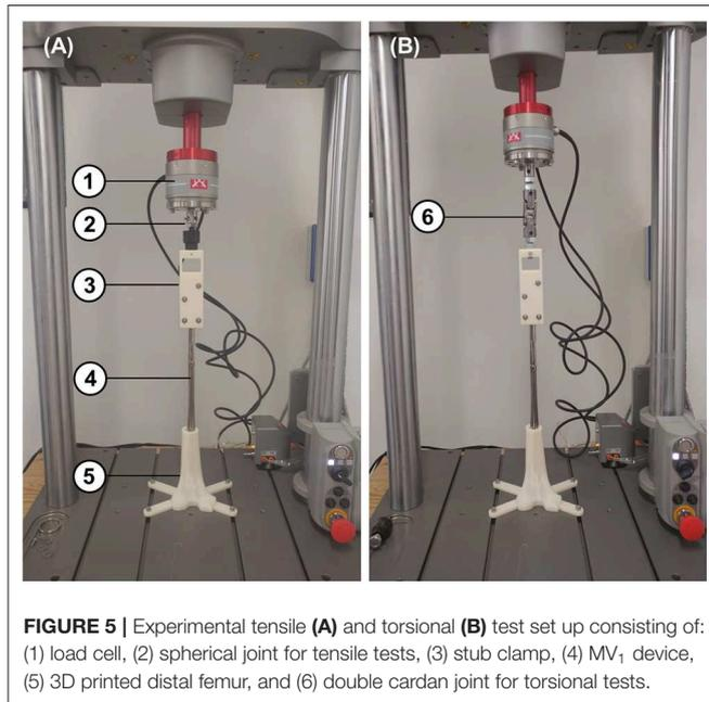
**FIGURE 5** | Experimental tensile (A) and torsional (B) test set up consisting of: (1) load cell, (2) spherical joint for tensile tests, (3) stub clamp, (4) MV<sub>1</sub> device, (5) 3D printed distal femur, and (6) double cardan joint for torsional tests.
