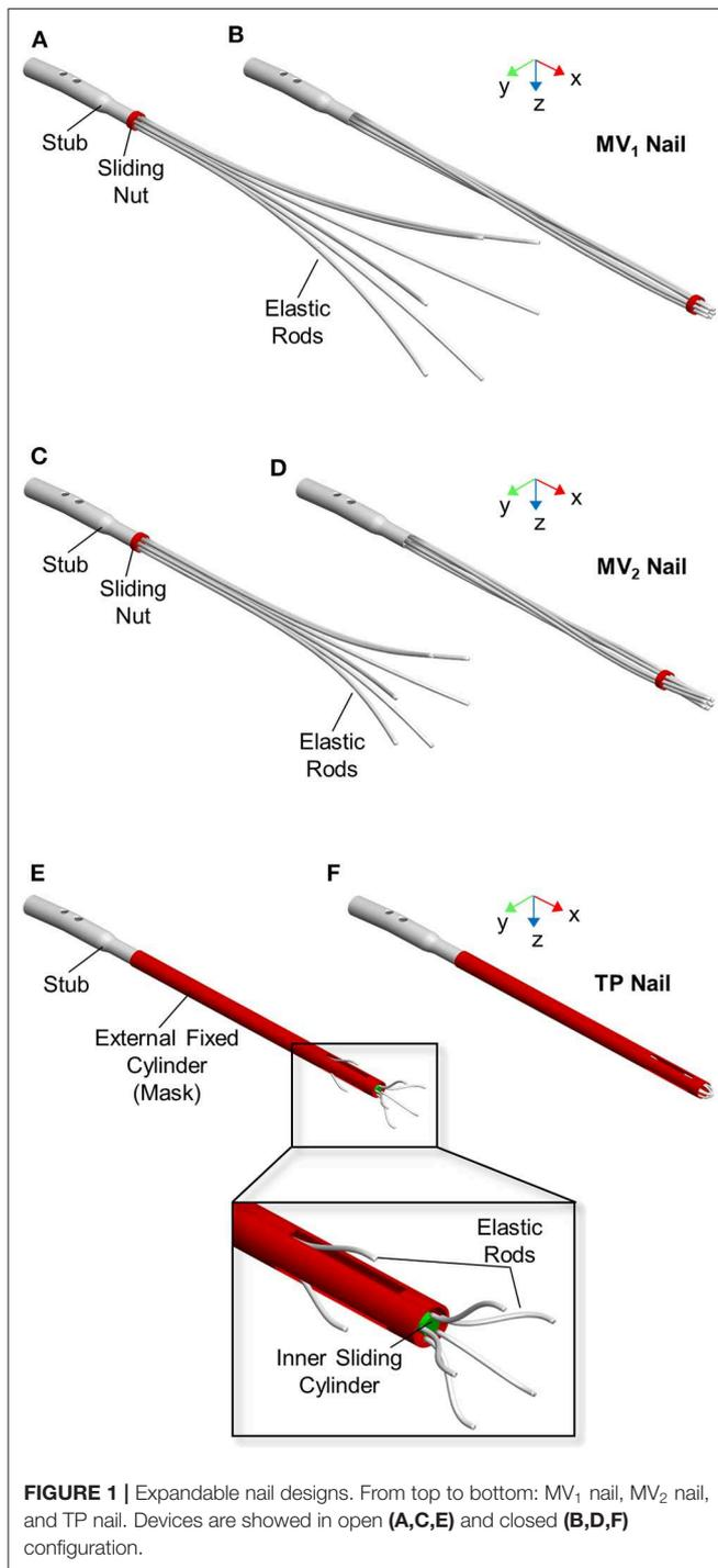
rods (circular cross-section with a diameter equal to 1.5 mm) departing from two different axial positions along a sliding inner cylinder (Figures 1E,F). In particular, the device is composed of 3 proximal rods and 5 distal rods. An external hollow cylinder, fixed to the nail stub, characterized by the presence of three radially equidistant slots, acts like a mask keeping the elastic
