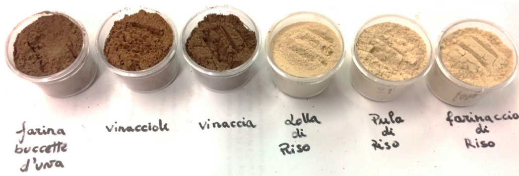
Figure 5. Mechanical treatment of wine and rice by-products from Agrindustria to obtain flours. Source: DISAT.
