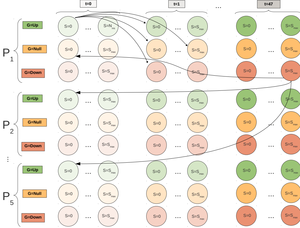
Fig. 4. Markovian model of the green system operation. Only some sample transitions, among all those possible, are reported.
