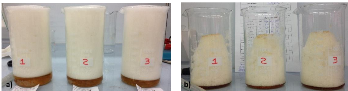
Figure 3 Foam produced with Foamin C ® protein foaming agent showing drainage a) and structural collapse (showed by all the foams produced) at the selected time interval of 180 minutes b).
