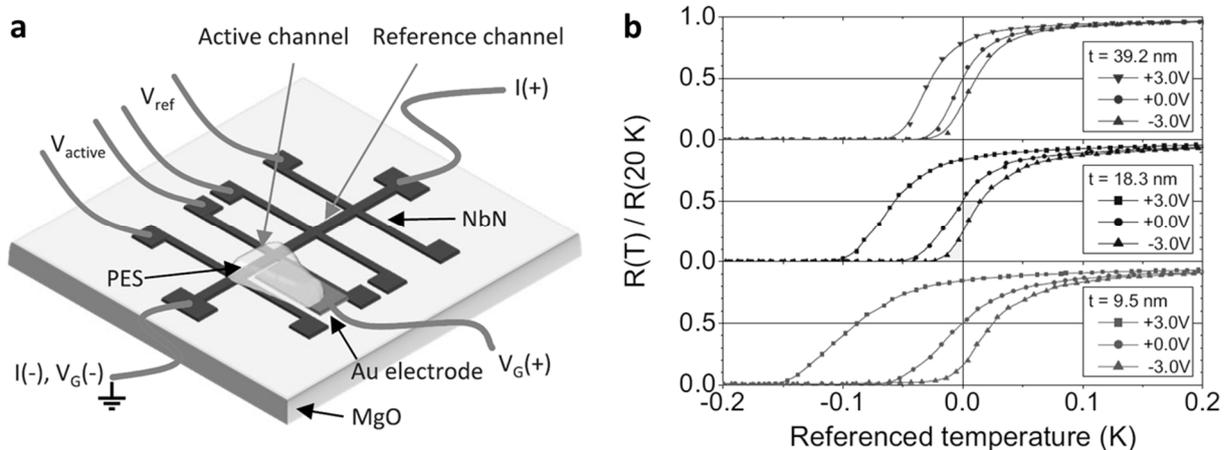
Figure 1: **a**, Sketch of a NbN-based EDL-FET in the dual channel configuration (active + reference). **b**, Normalized resistance of the active channel as a function of the temperature referenced to the midpoint of the ungated transition, for different applied gate voltages and film thicknesses. Adapted from Ref. 9.
