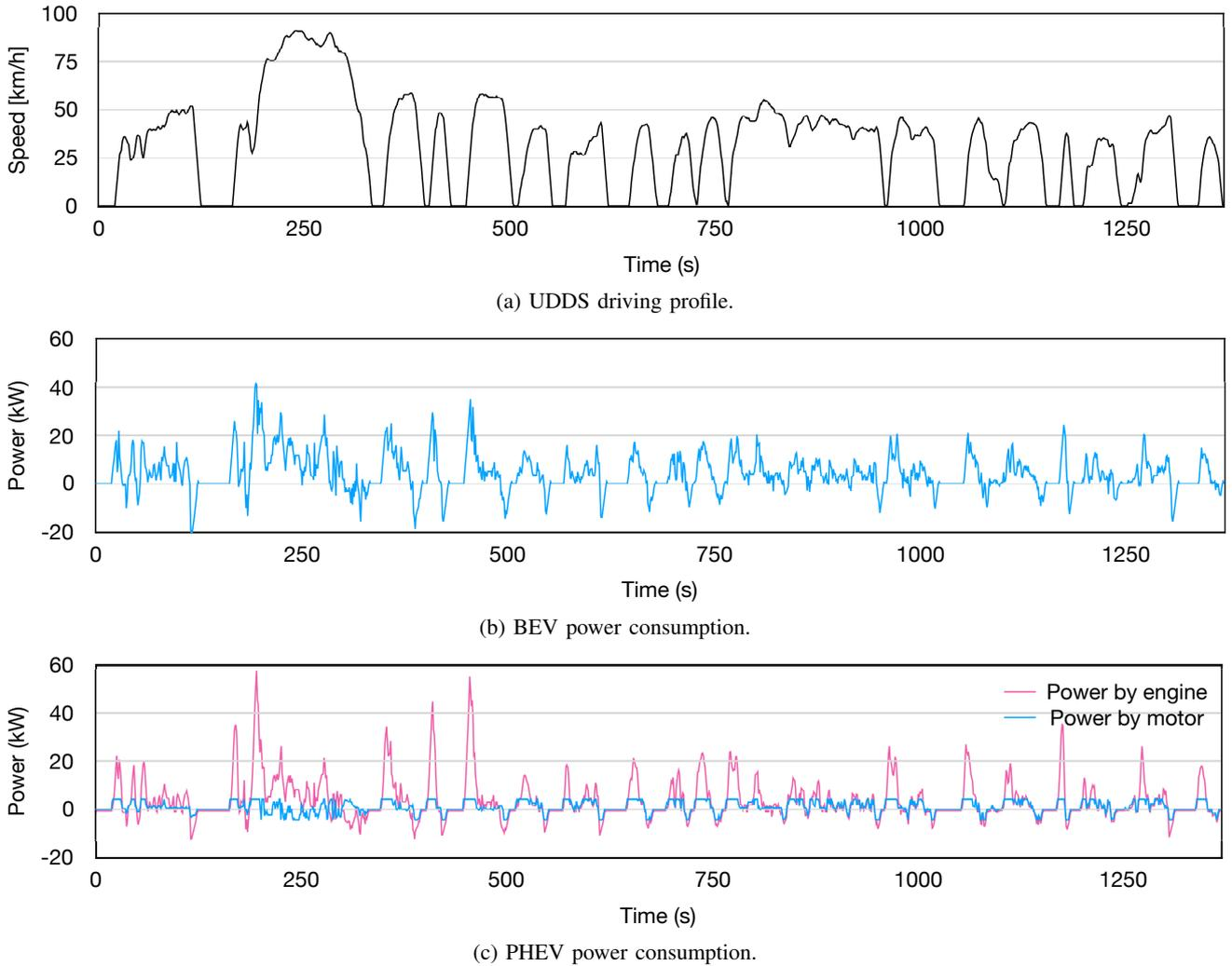
Fig. 2: Simulation results of the UDDS test cycle.
