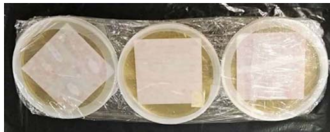
Figure 2. R. mucilaginosa contaminated sheets treated with Thymus vulgaris oil at time 0 and wrapped in polyethylene film.
