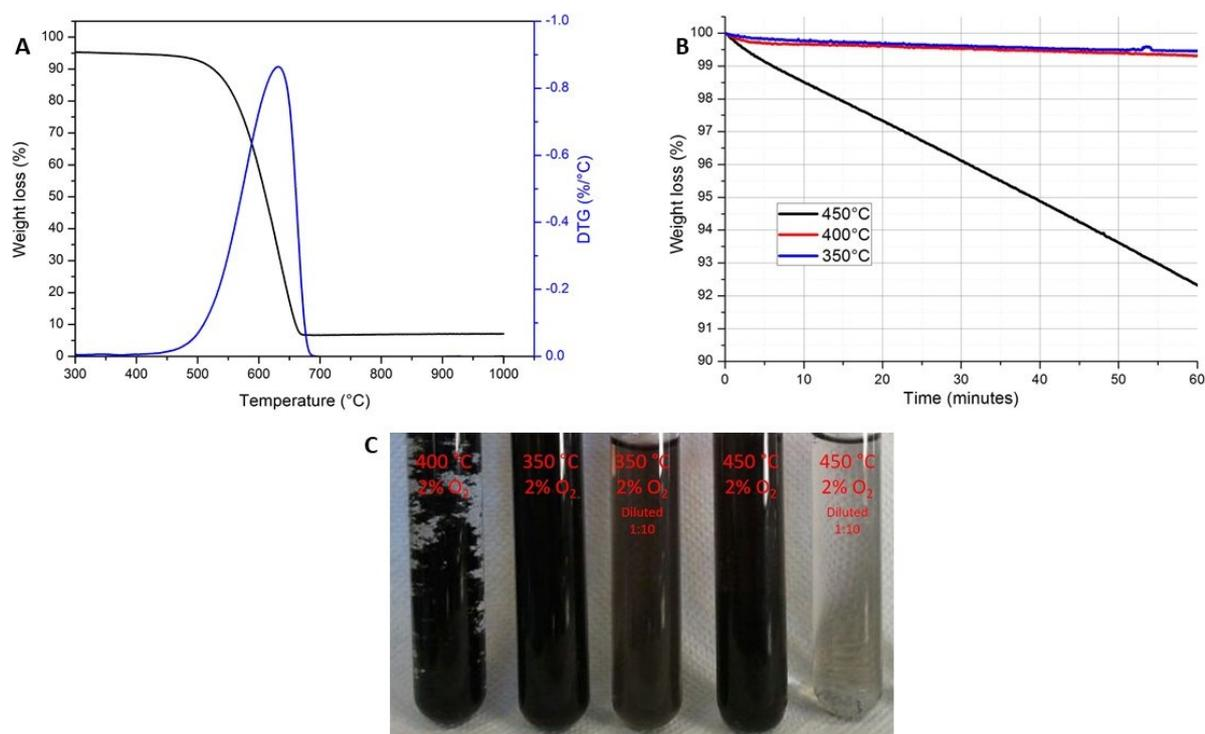
**Figure 1: A) TGA curves and derivative curves (DTG) of CNTs with a ramp of 5°C/min flux of 2% O<sub>2</sub> 98% Ar; B) Isothermal thermal gravimetric analyses at different temperatures (350°C, 400°C and 450°C); C) Dispersion of CNTs in water after isothermal treatment (some of the solutions are diluted 1:10 to better observe the degree of dispersion)**
