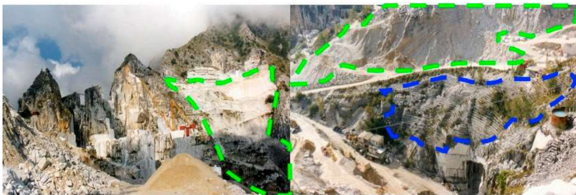
Figure 14. Carrara marble quarry basin: open pits and Ravaneti (green dashed lines). Some of the historical Ravaneti (blue dashed line) have been used as a base for the internal roads in quarrying areas.
