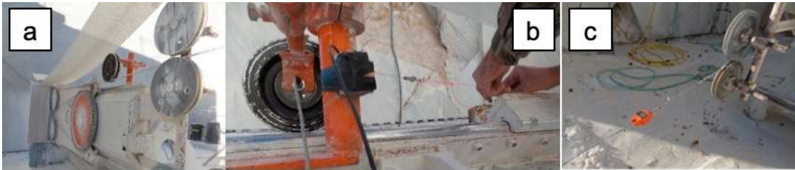
Figure 7. (a) Positioning of the load cell on the Apuania Corsi MF 5000 machine. (b) Placing the draw wire encoder. (c) Installing the dynamometer for calibration.
