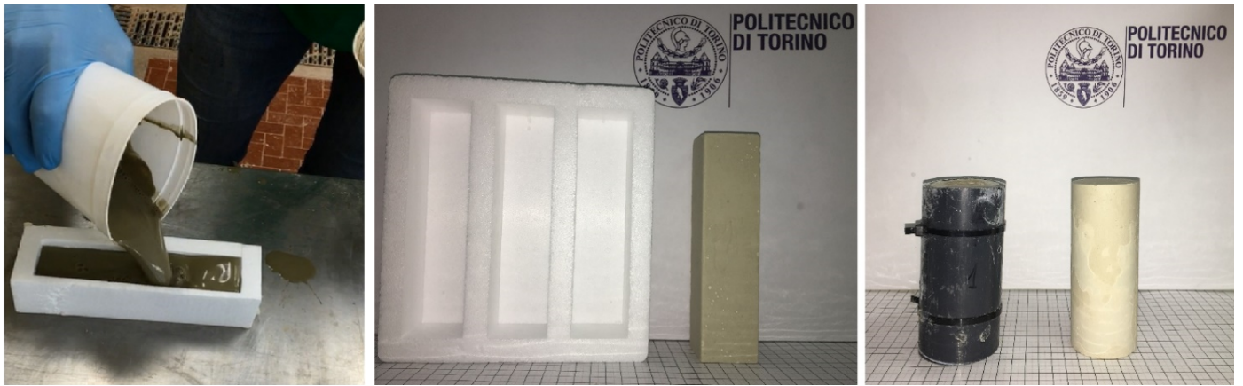
Figure 3: Casting of a prismatic sample, on the left. Example of used moulds and corresponding samples: cylindrical mould model on the right (internal diameter \phi = 52 mm, height = 130 mm) and prismatic one ( l = 40 mm, height = 160 mm) in the centre. The squares on the base background are 1\text{ cm}^2 .
