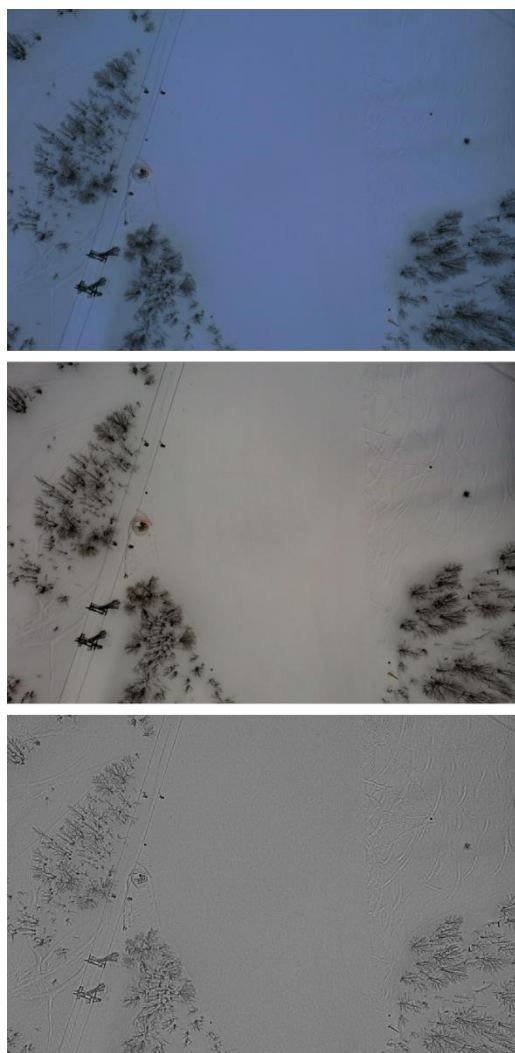
Figure 7. Example of image editing: the original image acquired by Mavic 2 Pro (upward), the with balance application (in centre) and the use of the Wallis filter (below).
