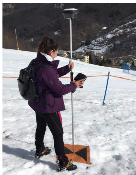
Figure 4. GCPs measurement with RTK approach.
