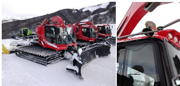
Figure 6. The snow groomer (on the left) and the installation of the antenna on the top of the vehicle.
