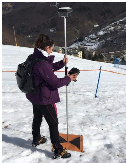
Figure 4. GCPs measurement with RTK approach.
