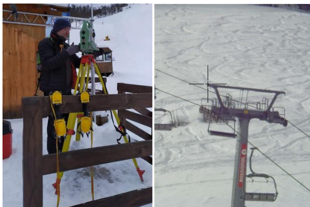
Figure 5. Detail survey with the total station.
