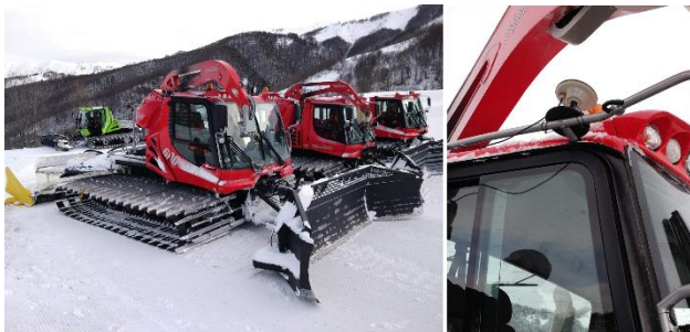
Figure 6. The snow groomer (on the left) and the and the installation of the antenna on the top of the vehicle.
