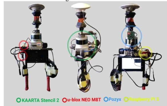
Figure 1. The multi-sensor platform which integrates: the KAARTA Stencil 2-16 MMS, two u-blox NEO M8T GNSS receivers, the Pozyx UWB and the Raspberry Pi 3 Model B+.
