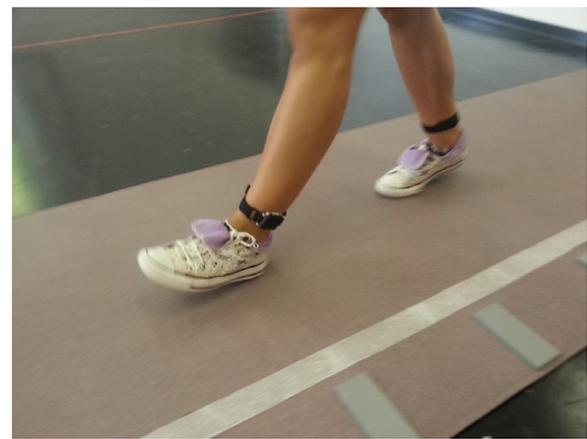
**Figure 1** Subject wearing two MIMUs attached above the ankles and walking on the instrumented mat used as gold standard for MIMU based estimates of gait spatio-temporal parameters.
